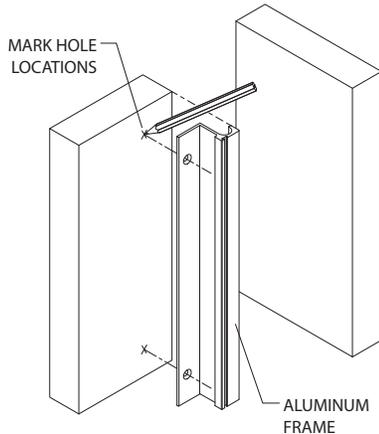
1. Install the architectural joint system on a level wall surface. This may require leveling to raise the tops of the frames.
